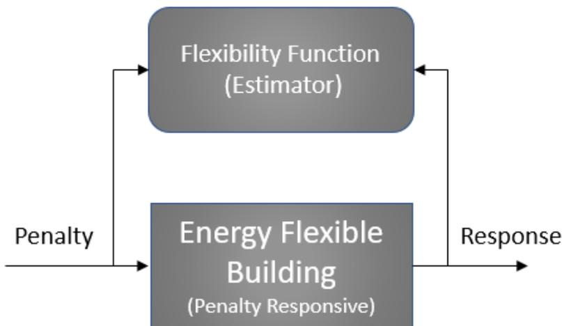
Figure 5.1 Signal flow for estimating a Flexibility Function of an energy flexible building responding to a Penalty signal.
