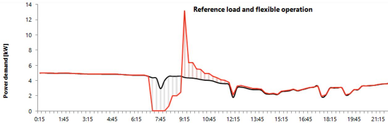
Figure 6.12 Reference load (black) and flexible operation (red) for a single downward flexibility event.
