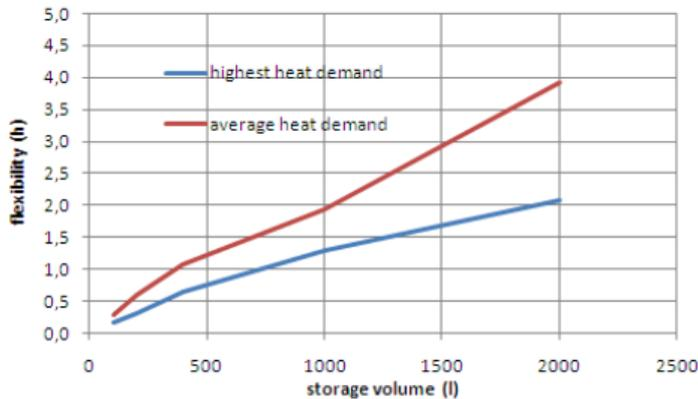
Figure 4.6 Flexibility as a function of the TES volume ( $\Delta T=10K$ ) (Six et al., 2011).
