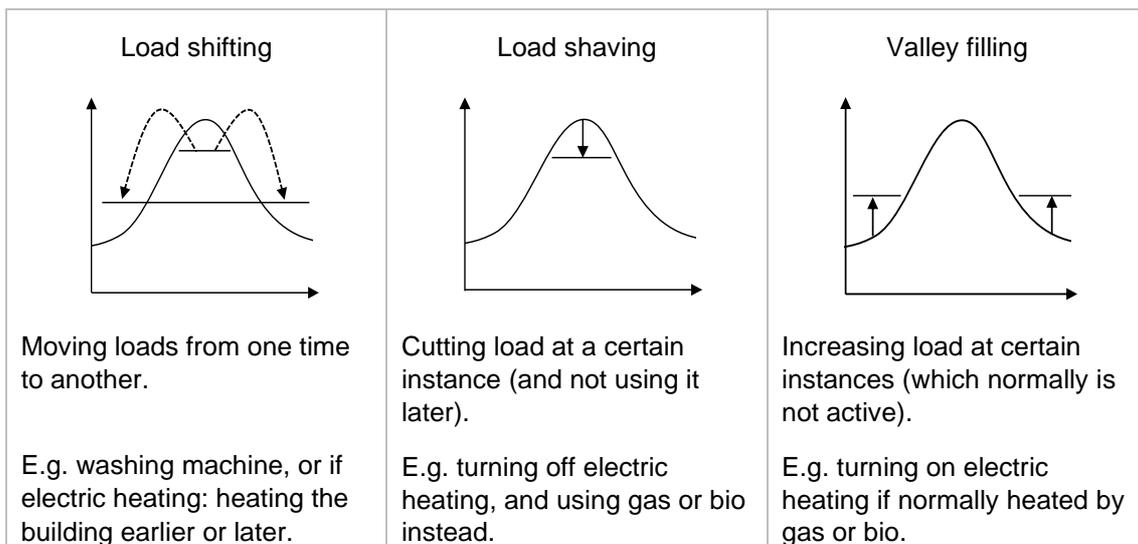
Figure 4.2 Flexible mechanisms: load shifting, load shaving and valley filling (Linberg, 2019).
