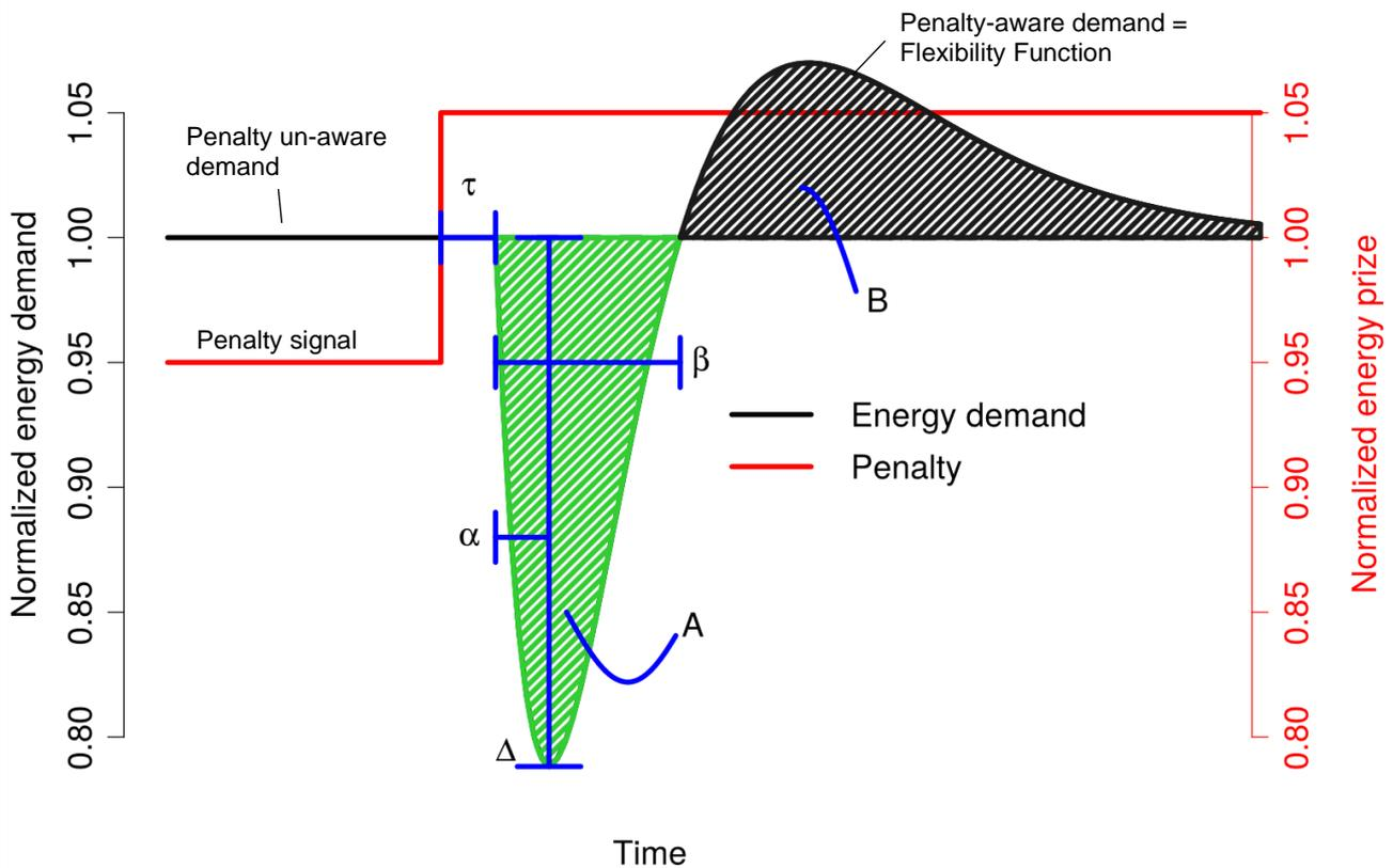
Figure 5.2 The expected response of some energy flexible buildings (without any prior knowledge regarding changes in the Penalty signal) exposed to a step increase in the Penalty signal, termed as the Flexibility Function.
