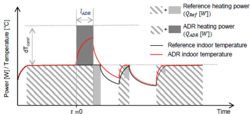
Figure 4.4 Scheme of the simulation experiment used to quantify the available storage capacity and the storage efficiency (Reynders, 2015).
