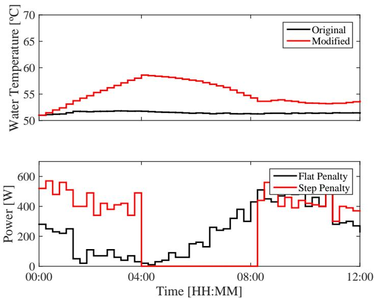
Figure 6.8 Water temperature (top graph) and power consumption (bottom graph) for both Penalty signals when the initial water temperature is 51°C. The black line always represents the values of the original water heater, the red lines the modified values caused by introduced block pulse/step penalty.
