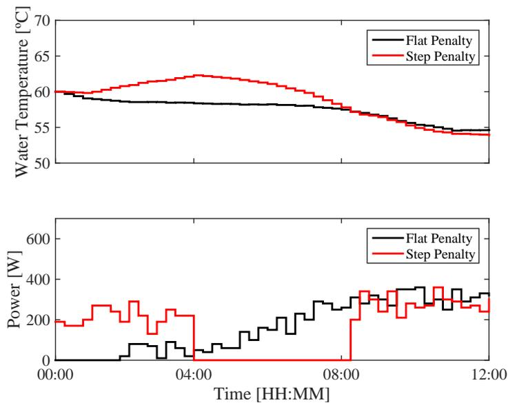
Figure 6.9 Water temperature (top graphs) and power consumption (bottom graph) for both Penalty signals when the initial water temperature is 60°C.
