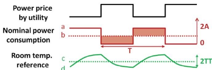
Figure 4.5 A hypothetical example which illustrates the flexible power signal (a), fluctuating between 0 and 2A around the nominal power (b). The shaded areas show the maximum energy varied to nominal value that can be tolerated by the system. (Tahersima et al., 2013).
