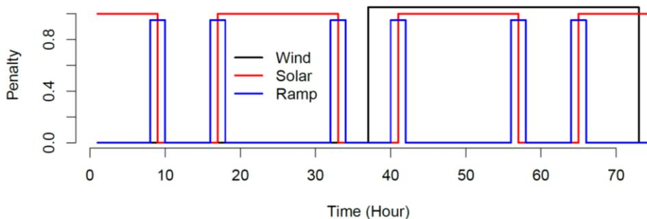
Figure 5.7 The Penalty signals from Figure 5.6 are simplified into more operational binary Penalty signals designed to obtain energy flexibility from the buildings when needed by the energy networks (Junker et al., 2018).
