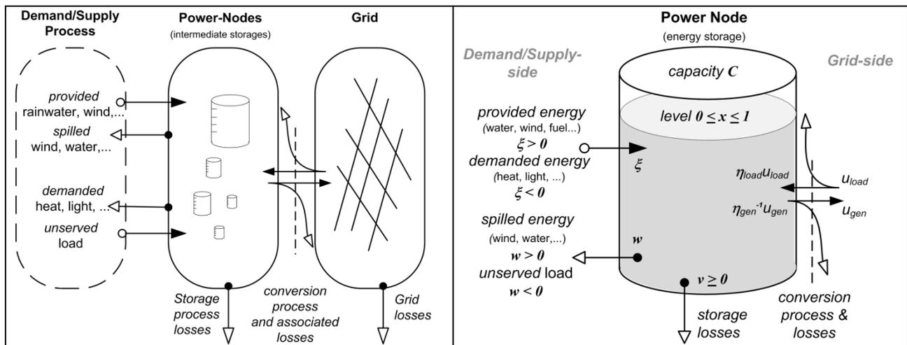
Figure 4.3 Power node domains (left) and notation for a single power node (right) (Heussen et al., 2012).
