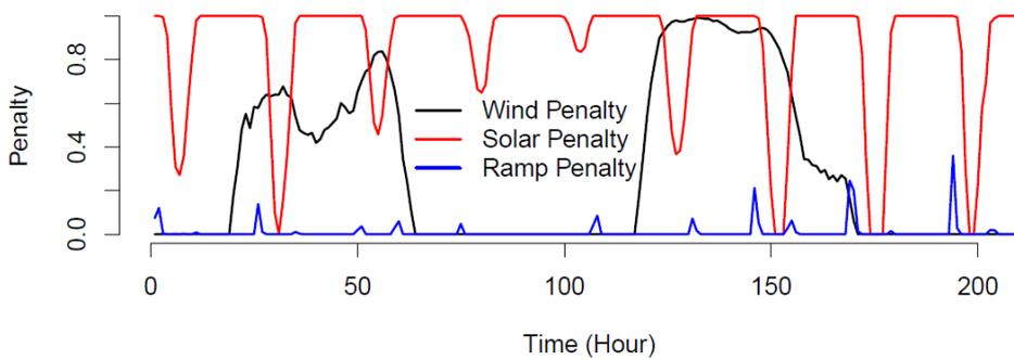
Figure 5.6 Penalty signals based on wind and solar power production in Denmark during 2017. Ramp penalty based on consumption in Norway during the same period (this situation is also typical for district heating systems) (Junker et al., 2018).
