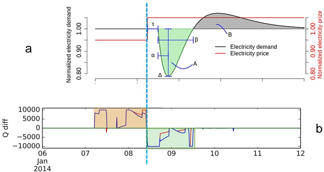
Figure 6.1 In the bottom graph (6.1b) an example is shown of the anticipation effect of energy demand in Watt as obtained when optimal predictive control of the building heating system is responding to a step change in price, introduced by dashed line coming from the top graph (6.1 a), and compared to the change in energy demand obtained by a non-predictive controller (6.1 a - top graph).
