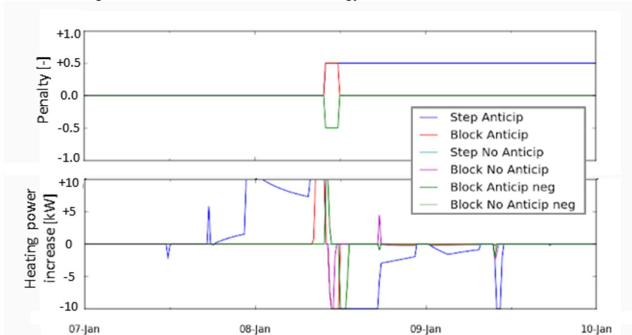
Figure 6.16 Evaluation of proposed penalty functions on a 2-zone building model, representing a typical Belgian detached single family dwelling constructed from 1990 to 2005 and equipped with radiator heating.
