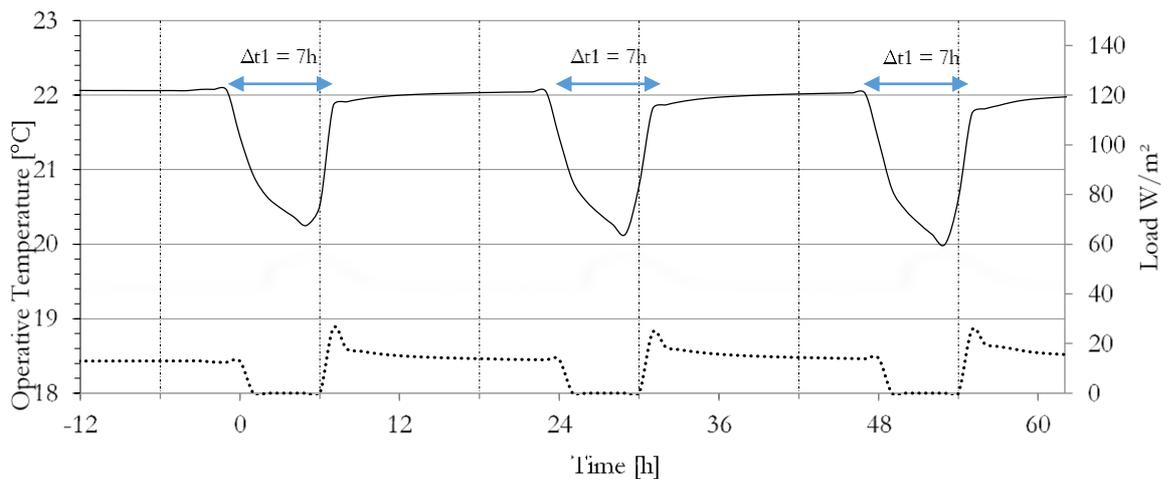
Figure 6.15 Periodicity and consecutive events, turning off the heating system every 24 hours: Top graph (full black line) shows the changes in the operative temperature while the bottom graph (black dotted line) shows the load changes.
