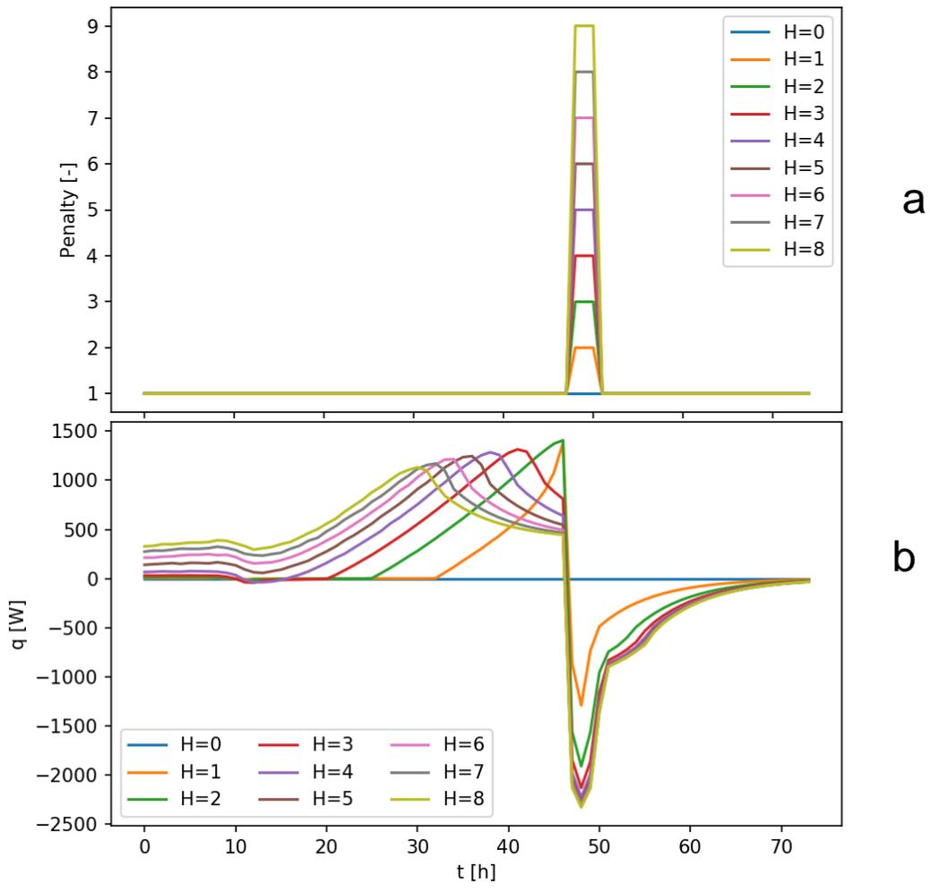
Figure 6.4 Impact of increasing amplitude of the penalty function (top) and the change in heating power profile compared to the flat price scenario (bottom).
