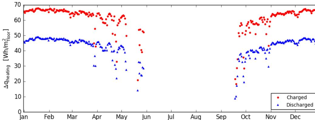
Figure 6.2 Influence of the outdoor conditions on the shiftable energy amount of A (red) = “charged” or “overheated” building by increasing the set-point by 2°C, and B (blue) = “discharged” or “cooling down” phase of the building - the transition season shows high variable values
