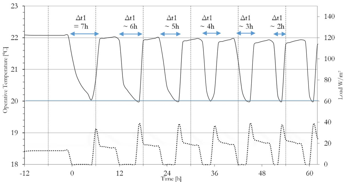
Figure 6.14 Periodicity and consecutive events, turning off the heating system every six hours: Top graph (full black line) shows the changes in the operative temperature while the bottom graph (black dotted line) shows the load changes.
