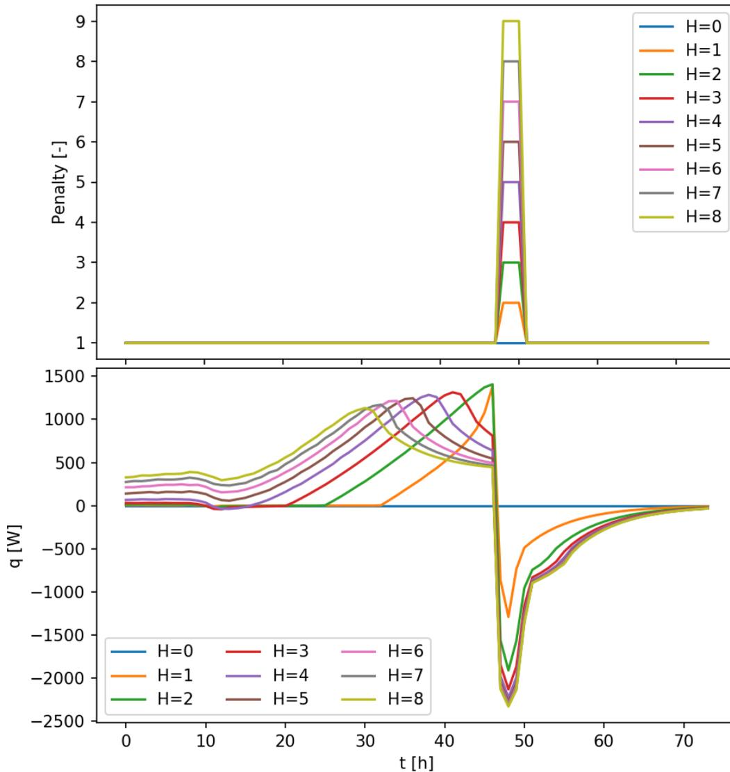
Figure 5.4 Impact of increasing amplitude of the Penalty signal (top) and the change in heating power profile using a MPC strategy compared to the flat price scenario  $H=0$  (bottom) (Jensen, et al., 2019). See also Section 6.3.3.
