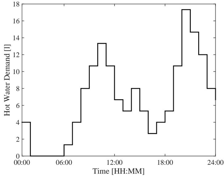
Figure 6.6 Hot water demand profile for four users (total hot water consumption of 160 litre per day).
