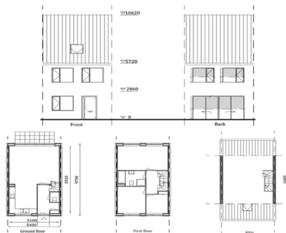
Figure 46 Layout of a typical Dutch terraced house, showing different floors, front and back view of the building. All dimensions are in mm.
