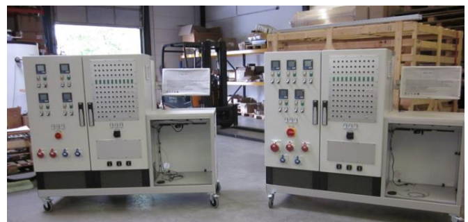
Figure 62: Central module with patch panel and electric energy balancing
