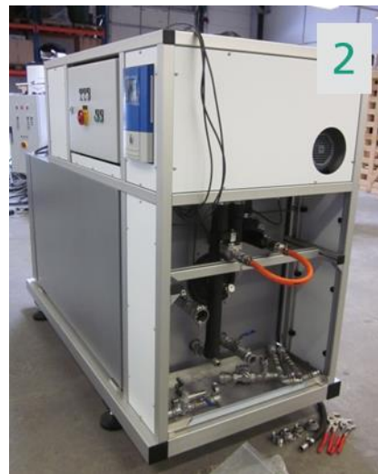
Figure 57: Submodule potable water
